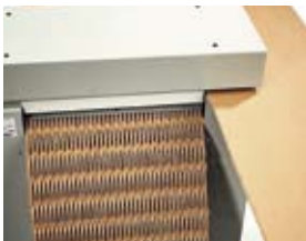
Cutting and perforation in one cycle. The end result is self-produced, high-quality packaging material.
